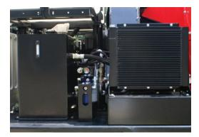
Easy-to-monitor hydraulic system Designed for efficient operation and service, the hydraulic system gauges are highly visible. Filter change and other routine maintenance can be performed at ground level.
