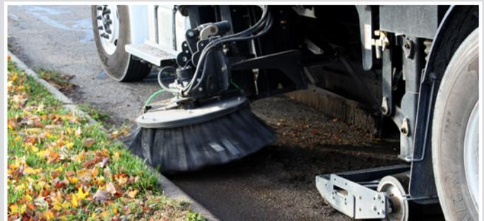
Brick said the model he was using had dual sweep capability, which is more effective picking up debris and leaves on city streets. "I can run both sweep brooms at the same time, cleaning a wider path," he said.
