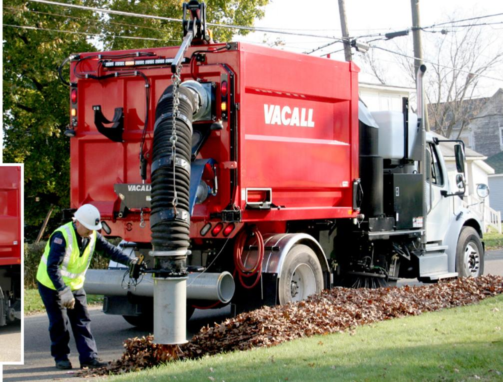
The new model also has two fixed position deflector brooms to keep debris from moving to the opposite side of the machine, feeding debris into the vacuum without the need for a mechanically driven transfer broom.
